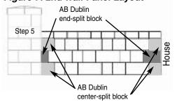
against the split block. We recommend installing the first two courses of the wall panel at the same time to ensure proper alignment.
