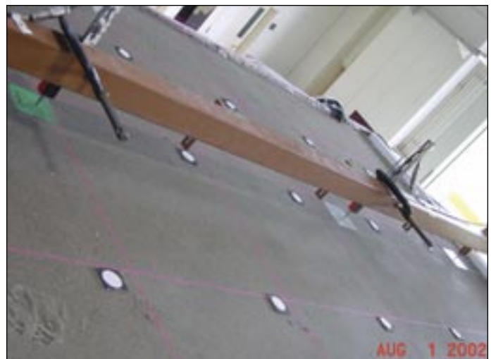
LVDT and Markers on the Backfill Surface
