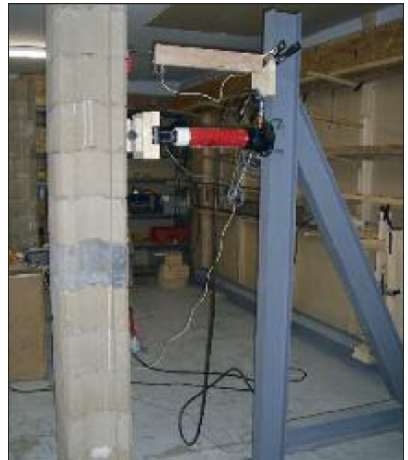
Hydraulic ram and frame assembly for AB Fence Post flexural test.
