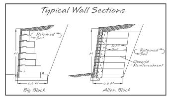
So, with the help of the local Allan Block Producer, Reading Rock, Milestone asked Civil Design Professionals (CDP) to prepare a value engineered preliminary design to be submitted for approval to BFS Engineers. The preliminary design consisted of AB Classics and geogrid resulting in an installed cost that was approximately half of the big block walls.
