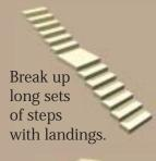
Drop in a turn and landing to break the stair line.
