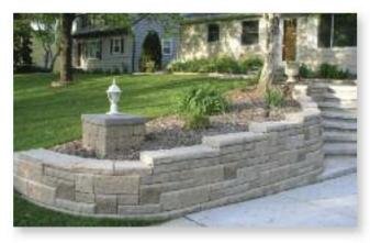
Another added benefit to using curves, is how easily they come together. In fact, most curved walls can be built with no cutting involved, making them simple to build.
