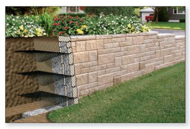
AB Reinforcement Grid is biaxial (strong in both directions) and can be simply rolled out along the wall. Other geogrids are uniaxial (stong in only one direction) and must be installed running from the front of the block to the back of the excavated area.
