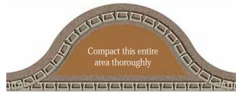
To prepare for the upper wall, this area will need to be compacted to 95% of Standard Proctor.
